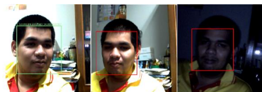
Figure 8 The results of face detection in a different light intensity.
