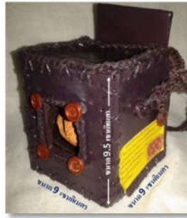
Figure 4 Bioplastic Packaging from Jackfruit Seed Starch sliding lid box type
