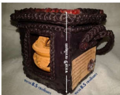
Figure 3 Bioplastic Packaging from Jackfruit Seed Starch cap lid box type
