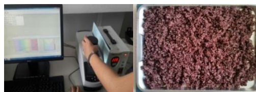
Figure 5 Color instant rice berry by the far infrared radiation drying at 2kW/m 2 .
