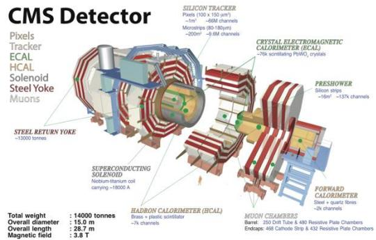
**Figure 1** Illustration with details of the CMS detector.
