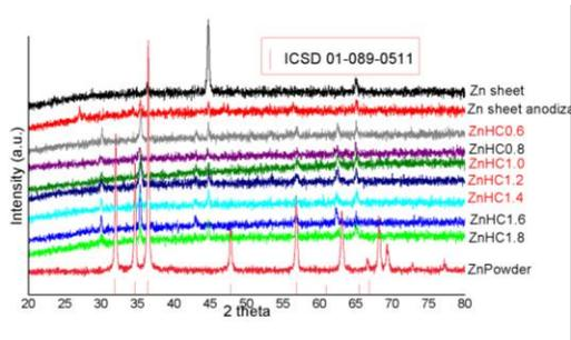
**Figure 1** XRD patterns of The Zn sheet substrates before anodization process using code Zn sheet and Zn sheet is anodization using code Zn sheet anodization. The samples were synthesized by hydrothermal under different the concentration of NaOH aqueous solution is 0.6g/L, 0.8 g/L, 1.0 g/L, 1.2 g/L, 1.4 g/L, 1.6 g/L and 1.8 g/L using code ZnHC0.6, ZnHC0.8, ZnHC1.0, ZnHC1.2, ZnHC1.4, ZnHC1.6 and ZnHC1.8
