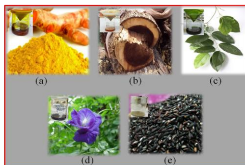
Figure 2 Photography of natural dye-sensitizer which are (a) the Turmeric (b) the saman bark, (c) Bai-ya-nang, (d) the Butterfly pea and (e) Black rice, respectively.
