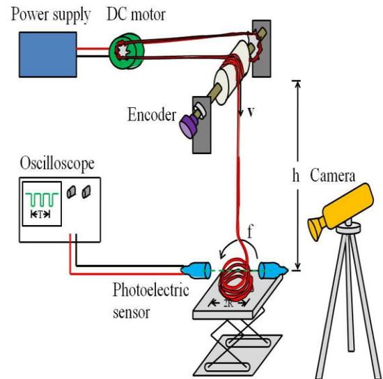
**Figure 2** Experimental setup for measuring the coiling frequency  $f$  of the rope fed from the height  $h$  with uniform velocity  $\mathbf{V}$ .
