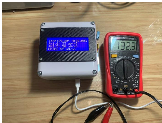
Figure 9 The measuring of minimum current usage
