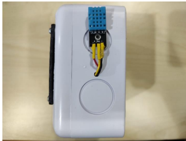
Figure 6 Side of real device with DHT11
