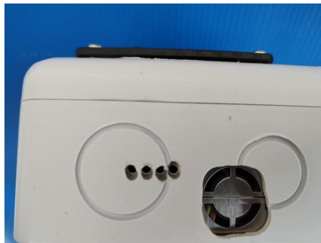
Figure 7 Side of real device with air vent of PMS7003
