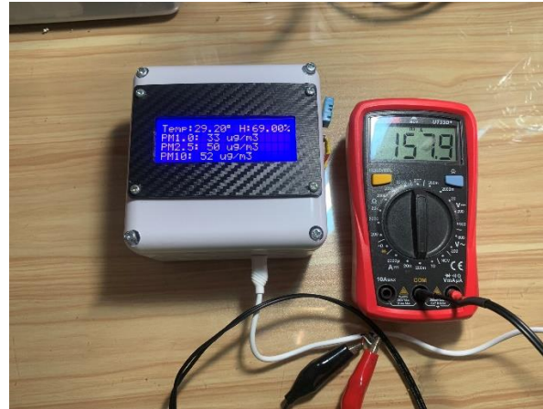
Figure 10 The measuring of maximum current usage
