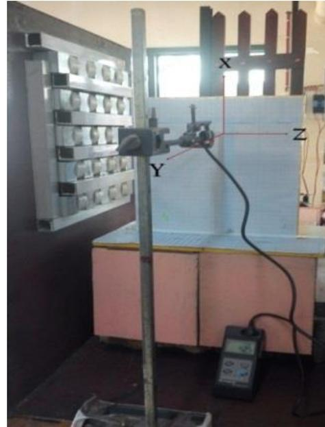
**Figure 2** Set up for measuring a magnetic field from a plate of 25 small permanent magnet cubes.
