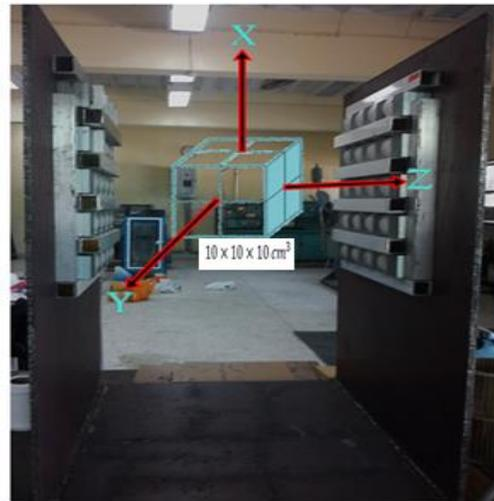
**Figure 3** A permanent magnet system with directions for measuring magnetic fields.
