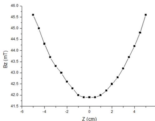
**Figure 6** Plot of a magnetic field in the z direction ( $B_z$ ) from the permanent magnet at distance ( $z$ ) from -5 cm to 5 cm.
