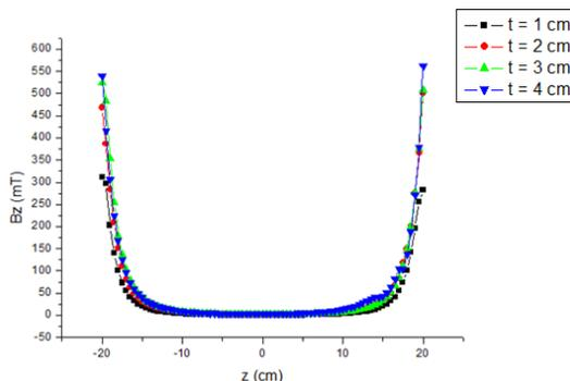
**Figure 5** Plot of a magnetic field in the z direction ( $B_z$ ) from two permanent magnet cubes with different thickness ( $t = 1$  cm, 2 cm, 3 cm and 4 cm) separated by a space 40 cm.
