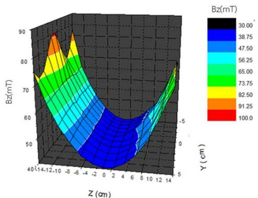
**Figure 7** 3D Plot of a magnetic field in the z direction ( $B_z$ ) on YZ plane from the permanent magnet at distance ( $z$ ) from -15 cm to 15 cm.
