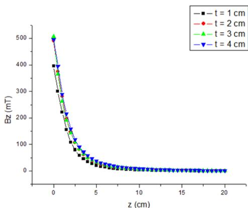
**Figure 4** Plot of a magnetic field in the z direction ( $B_z$ ) from a permanent magnet cube with different thickness ( $t = 1$  cm, 2 cm, 3 cm and 4 cm).
