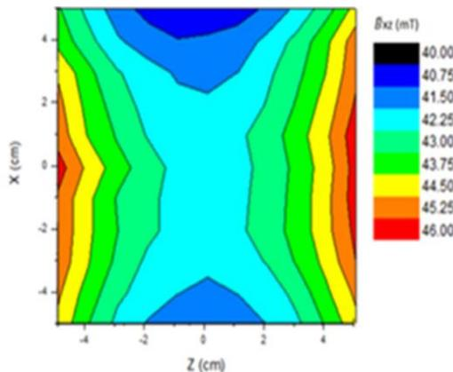
**Figure 9** Contours of the magnetic field on XZ plane at distance ( $z$ ) from -5 cm to 5 cm.
